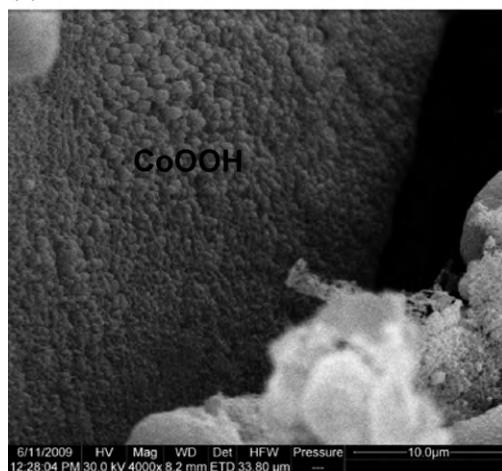
Fig. 12. SEM images of the cross-sections of the positive electrodes; area is close to the nickel foam and taken after testing: (a) Co-added cell, (b) CoO-added cell.
